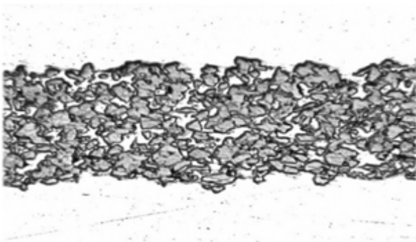
Figure 18. Typical micrograph of the meat of UMo-Al dispersion miniplate.
