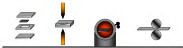
Figure 3. Mechanical-metallurgical steps of fabrication: Picture in frame assembly of fuel, welding, heating and rolling.
