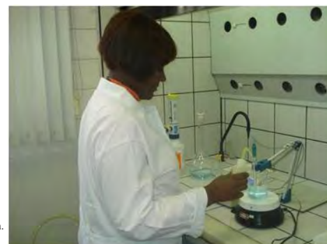
Figure 20. Davies & Gray potentiometric titration for uranium content determination.
