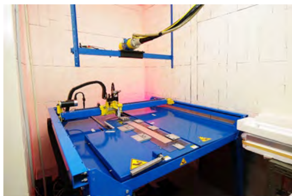
Figure 6. X-ray source, fluoroscope and automated tracing system (the aluminum fuel plate is located in the middle of table).
